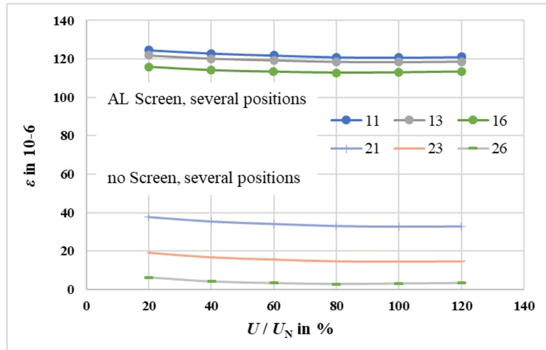
→ **Result with AL screen:** variation of the ratio error in different positions is reduced by a factor of 4 (uncertainty can be reduced)
