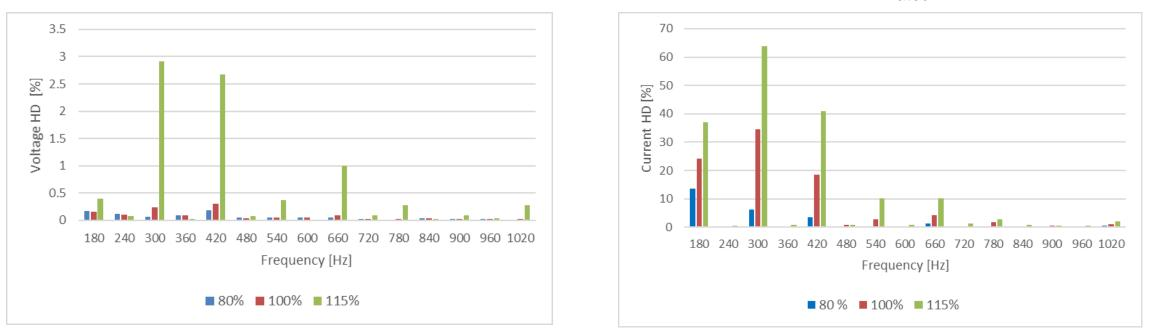
The distortion of 115 % case is higher than the lower voltage levels since the current are much more distorted combined with a non-negligible output impedance of the generator.
