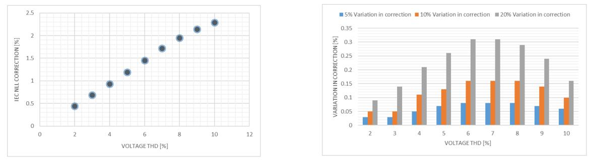
With less than 5 % error in the voltage THD, the maximum 1.3 % IEEE/IEC correction values in the present NLL measurements will be accurate to 0.1 %.
